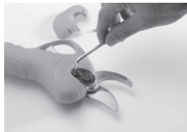
2. Remove the screws from the blade nut retaining buckle (this step is critical).
